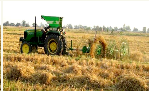
Field operation of tractor operated rake
